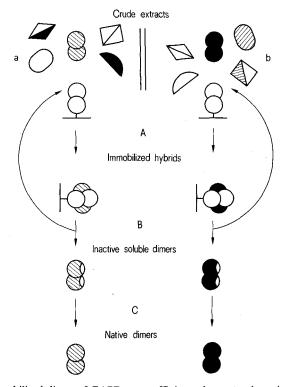
Immobilized dimer of GAPD as an affinity sorbent. A, adsorption of dimers existing in the crude extracts of different tissues (a,b) with subsequent washing from unbound proteins. B, incubation under the dissociating conditions and washing of the sorbent, which may be used repeatedly. C, reactivation of the soluble dimers. The figures of different shape refer to various proteins.
